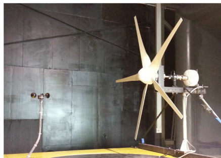
Figure 1: Wind tunnel test for torque and electric power measurements.
