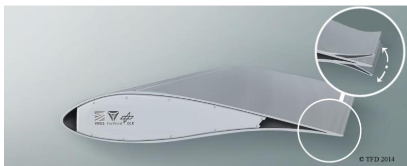
Figure 1: Airfoil equipped with a morphing trailing edge
