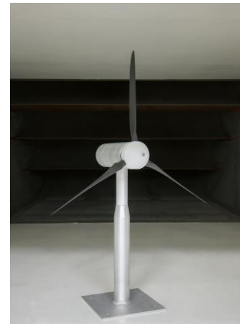
Fig.1: Model wind turbine, rotor diameter D=58\text{cm} .
