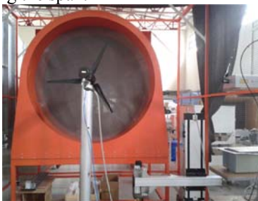
Fig. 1: Experimental setup; Open-jet wind tunnel and the PIV system
