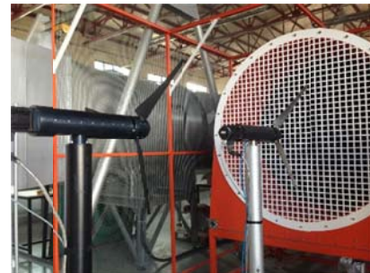
Figure 2 - Two model horizontal axis wind turbines positioned at the exit of open jet wind tunnel.
