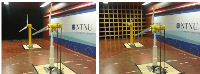
Fig. 2. Turbine models exposed to low (left) turbulence inflow and high (right) turbulence inflow
