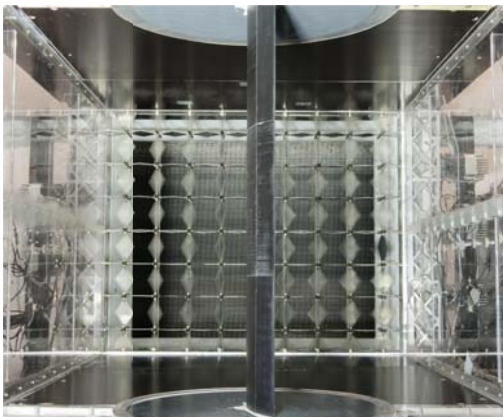
Fig. 1 Self-adaptive camber profile mounted in the closed test section of the wind tunnel downstream of the active grid.
