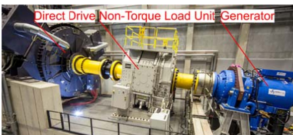
Fig. 1: Nacelle Test Bench
