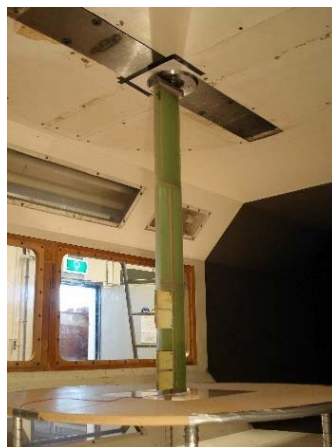
Figure 1: The adaptive blade used in [1] to demonstrate the potential of active load reduction
