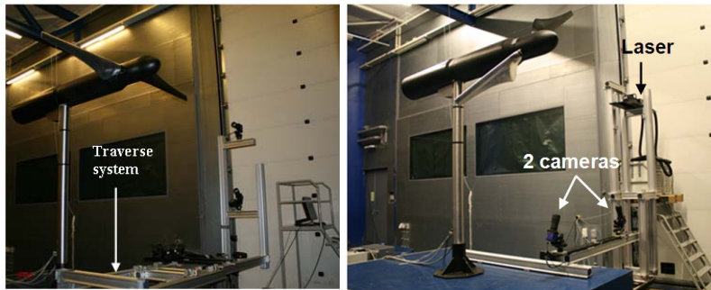
Figure 2: Chordwise (left) and spanwise (right) measurement setups.
