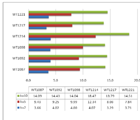
Figure 5: Wind Speed Turbulence Coefficient over the total length of wind speed data
