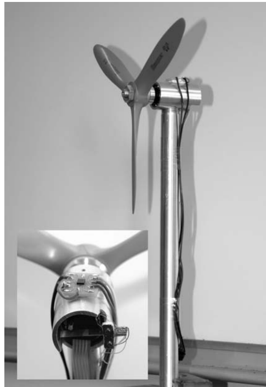
Figure 5: Improved setup of the turbine model: A smaller motor with a smaller encoder are used. The torque sensor is placed in the nacelle since no prolongation of the drive shaft is needed.
