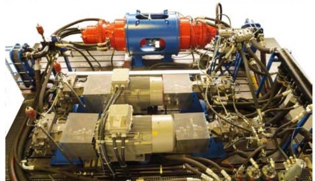
Figure 4: IFAS 1 MW test bench [5].
