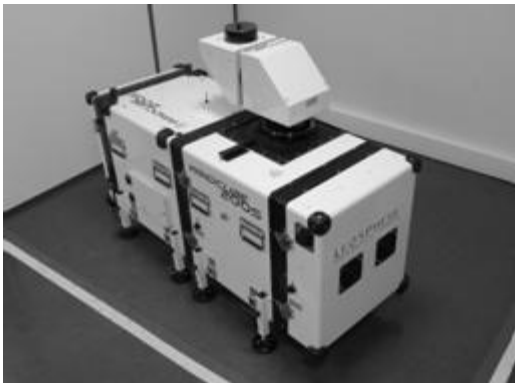
Figure 1: The long-range windscanner – the single device.
