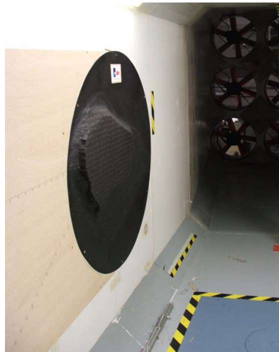
Figure 1: Model of the Bolund Island for wind tunnel testing
