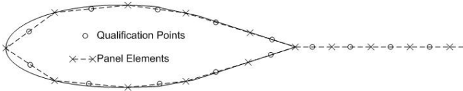
Figure 1: An example airfoil and wake modeled with linear panel segments of constant strength. Qualification points at which the potential is evaluated are also shown.
