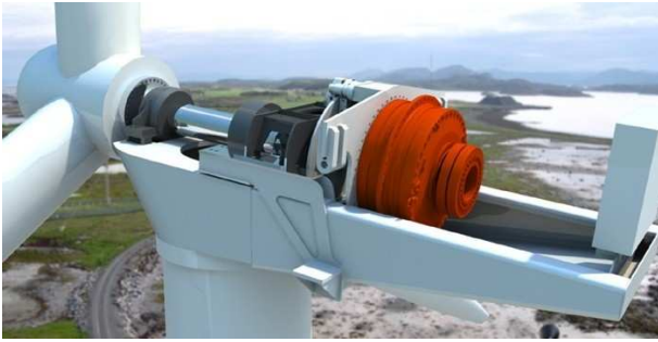
Figure 2: Chapdrive drive train solution for wind turbines [3].
