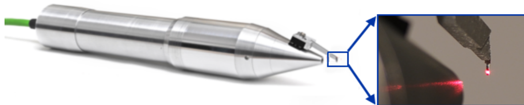
Figure 1: Design of the 2d-Atmospheric Laser Cantilever Anemometer with detailed view of the Cantilever.
