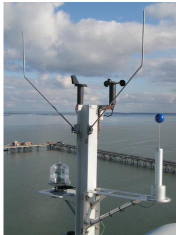
Figure 1: Sphere anemometer and cup anemometer installed on the nacelle of a near-shore wind turbine in the German Wadden Sea.
