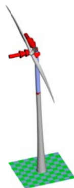
Fig. 1: Multibody model (SIMPACK) of a 2-bladed wind turbine (Source: Skywind).
