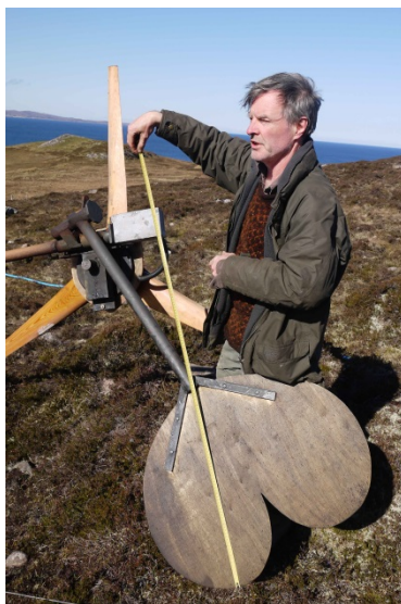
Fig. 1: Analysis of furling system performance by a) measurement of tail moment arm and b) power performance logging
