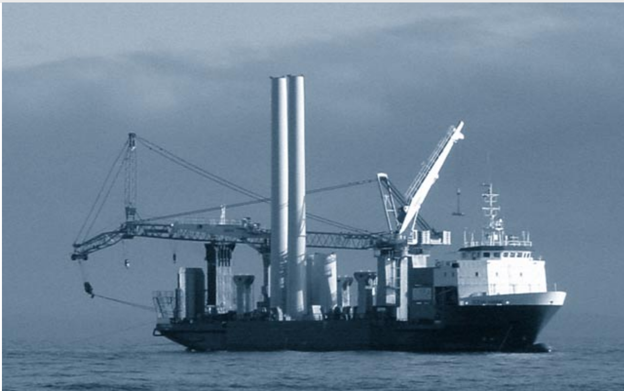
Installation vessel for offshore wind mills
