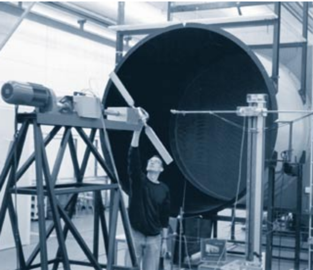
A model of a rotor placed in front of the open jet wind tunnel of Duwind
