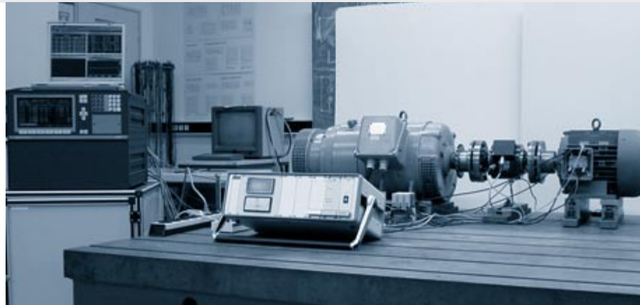
Test bench for wind converter drive train development
