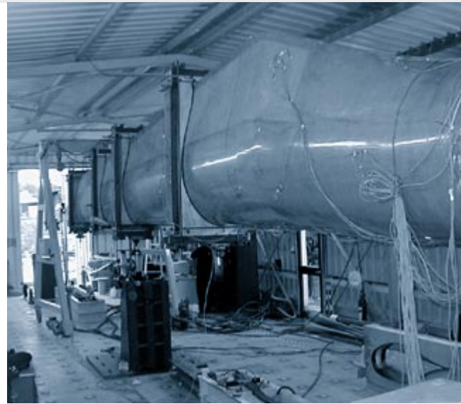
CRES laboratory for full-scale wind turbine blade testing
