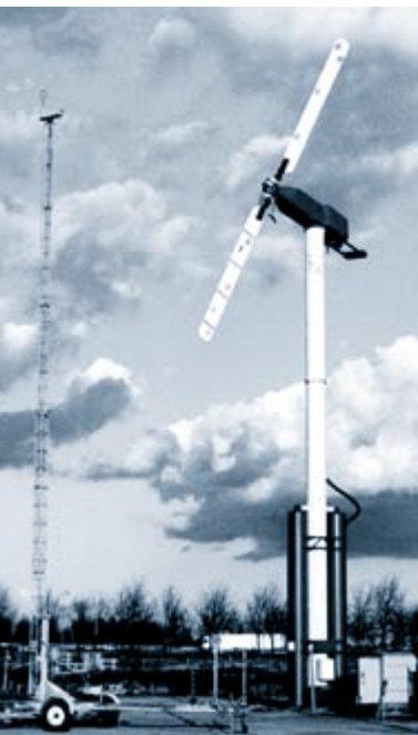
The experimental turbine for rotor research, with a tiltable tower to have easy access to the blades
