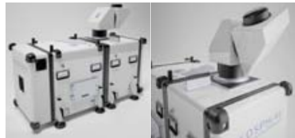
Figure 1: The long-range windscanner – left a single unit, right a fully steerable scanner head
