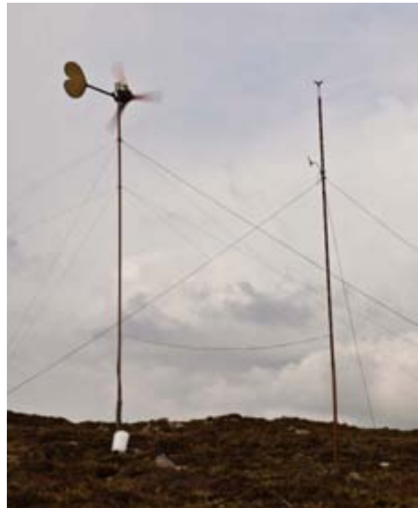
Figure 3: Data logging set up on the 1.8m diameter turbine.
