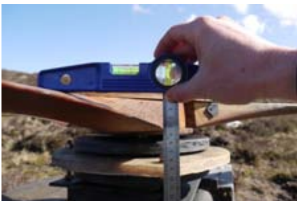
Figure 2: Measurement of the setting angle at the blade root using spirit level and ruler.
