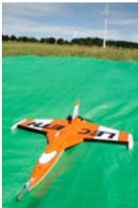
Figure 1: Instrumented UAV (wingspan, 800 mm) equipped with a seven-sensor fast response aerodynamic probe (diameter, 20 mm).
