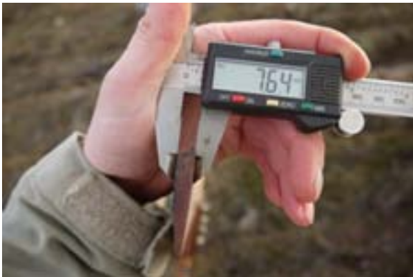
Figure 1: Measurement of the aerofoil thickness at the blade tip using digital callipers.
